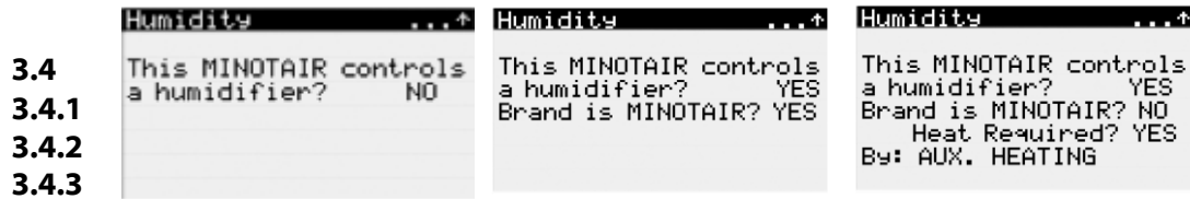
Figure 51 - Examples of options to adjust humidifier settings.
