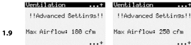
Figure 39 – Examples of options to adjust the maximum airflow.
