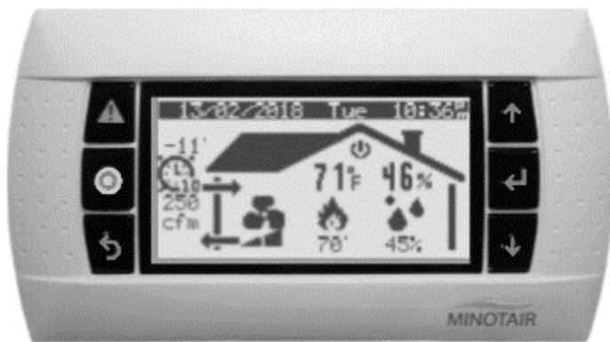
Figure 33 – Activation of the Virtual Bathroom Timer is done by pressing ⏪ and Ⓞ.
